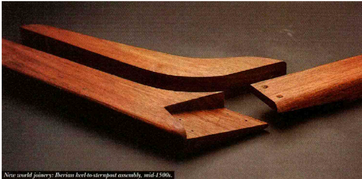
New world joinery: Iberian keel-to-sternpost assembly, mid-1500s.
